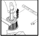
Open the door and remove the drainpipe
