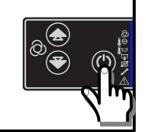
Switch on by a long pressing of ON/OFF button
