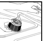
WHEN TANK IS EMPTY, REMOVE ALL FILTERS AND THE WASH ARMS BY UNSCREWING THE RETAINING NUT AND WASH THEM
